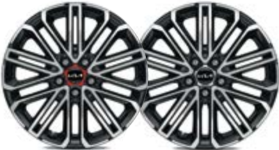
Alloy wheel 18". Bicolour, 7.5Jx18, suitable for 225/40 R18 tyres. 52910J7500PAC
