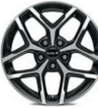
Alloy wheel 17". Bicolour, 7.0Jx17, suitable for 225/45 R17 tyres. 52910J7600PAC
